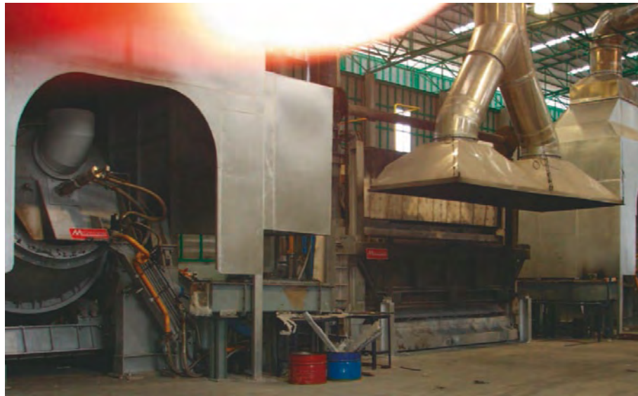
Two 5-tonne-capacity tilting rotary melting furnaces recently commissioned in Thailand
