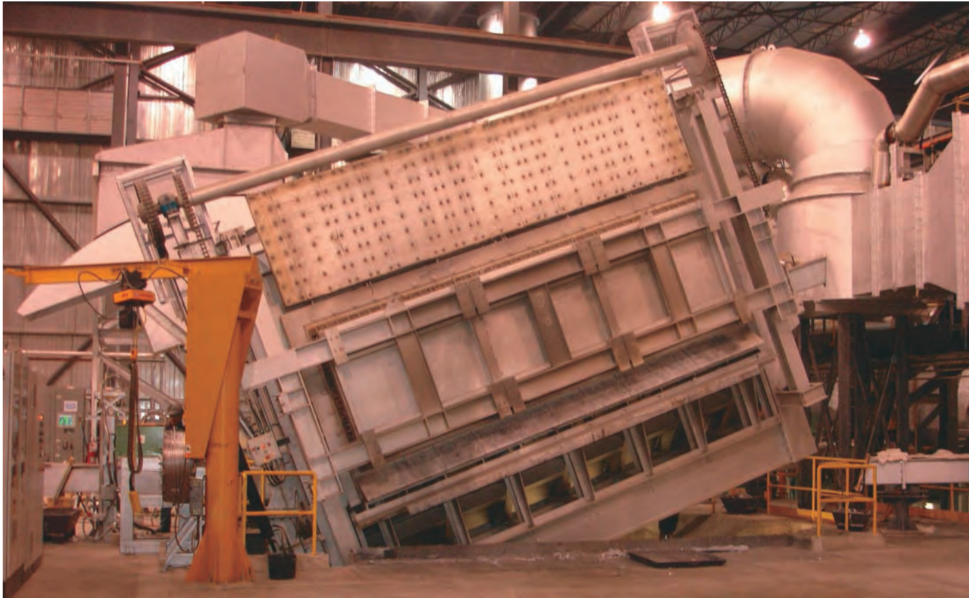
The contract for Metalco, Canada, also includes a 32 tonne tilting holding furnace
