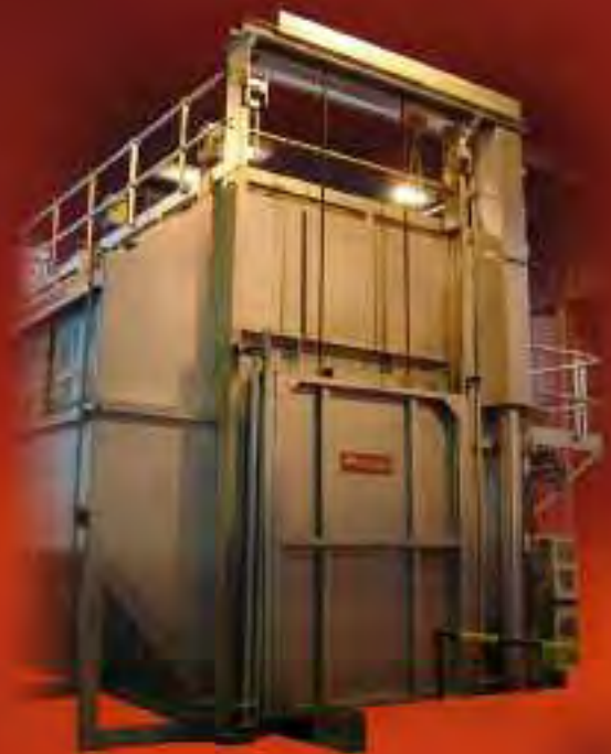
20t Batch Homogenising Furnace
