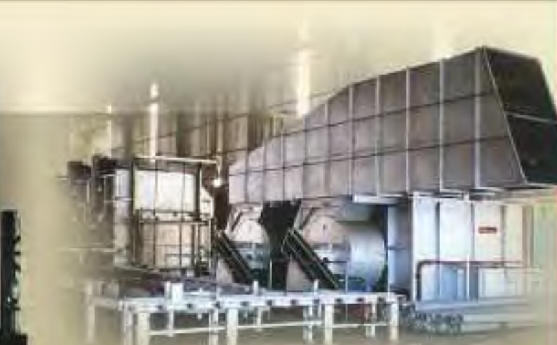
Bogie Type 20t Homogenising Furnace & Cooling Chamber
