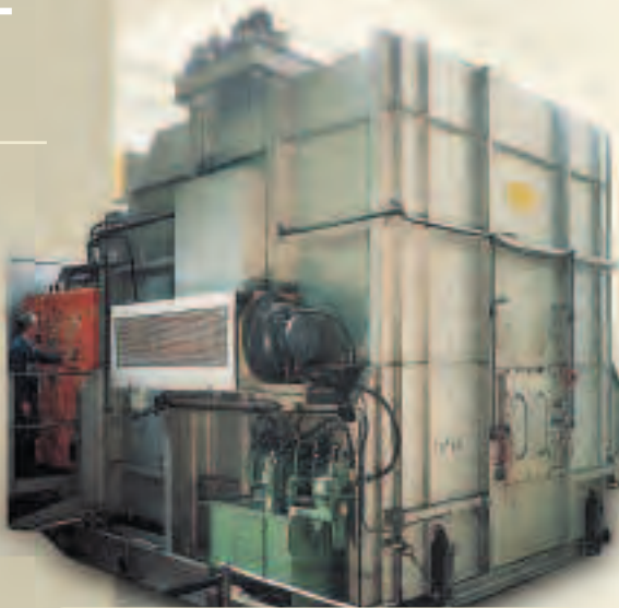
Forging & Extrusion Solution Heat Treatment Plant with Moving Furnace & Double Heated Quench Tanks
