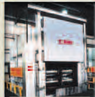
10t Foil Annealing Furnace with Nitrogen Atmosphere
