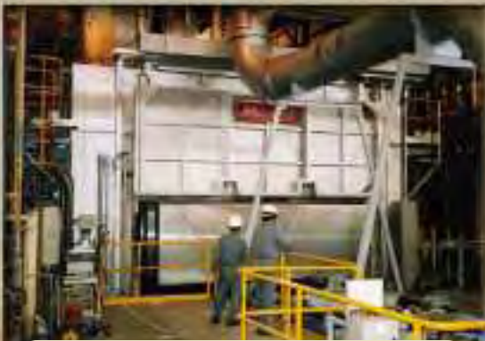
Continuous 40t/hr Slab Pusher Furnace with Charge and Extract Gear
