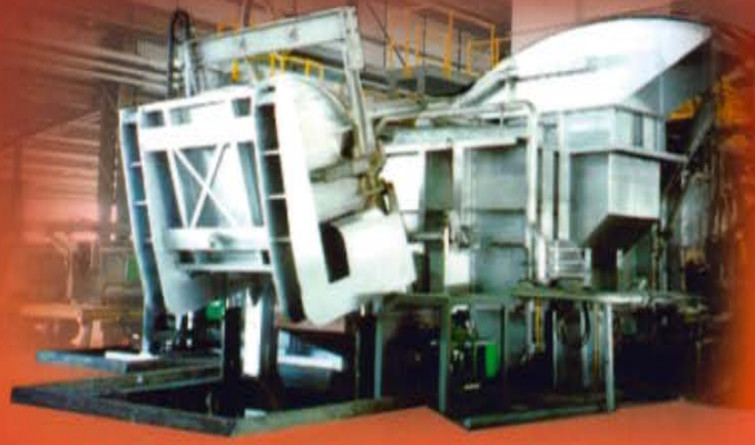
Hot Metal Crucible Tilt Machine for Furnace Filling
